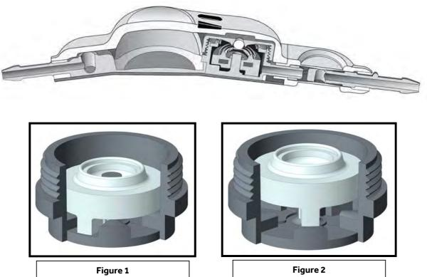
Example of a **Correct** rotor orientation
